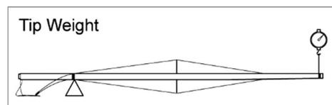
**H.4.7** **Mast centre of gravity height** shall be checked with any **halyards** fully hoisted and **rigging** pulled taut and tied to the **spar** as close to the **lower point** as possible.
